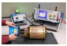
Testing an armature using the ZTX accessory and the ATF5000 commutator probe.
